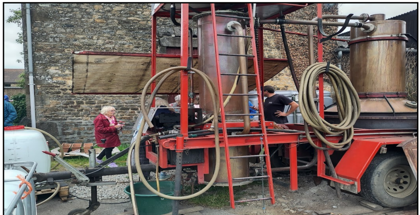
A mobile alembic: two vessels connected by a tube to distil liquids
